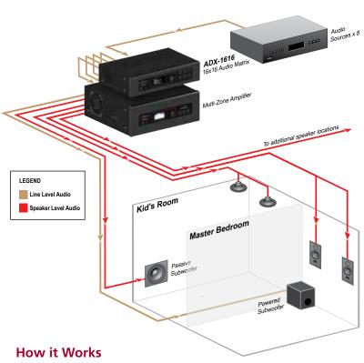
Designate any zone output as a lowpass sub out, and group it with a full range zone. The 2.1 zone group now functions as one zone, responding to group switching and group volume commands in tandem.
