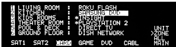
The Zone view allows the user to see the name of the locations and the sources. Asterisk (*) indicates that one or more of the Wallplates in the zone has been assigned a different source than the one shown.
