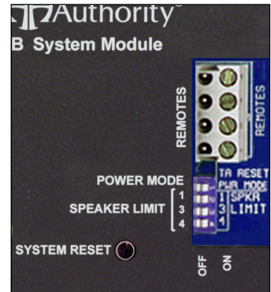
Figure 58. 980 Speaker Limit Switches.
