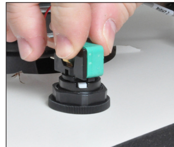
Figure 52. Inserting switch into PSB.
