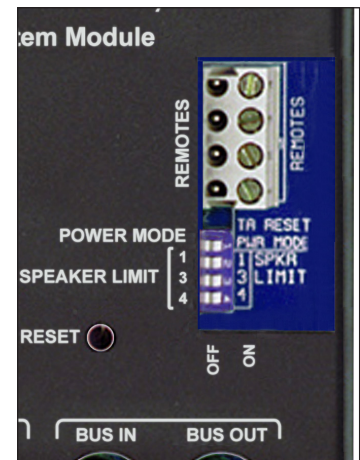
Figure 33. 980 speaker limit switches.
