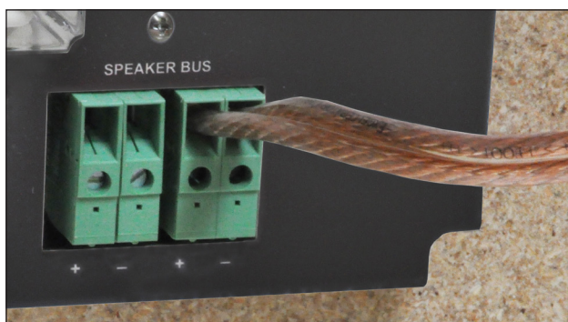
Figure 28. High-Power Speaker Bus using 12 gauge speaker cabling.
