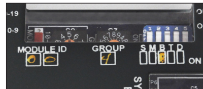
Figure 13. The first module in group 4 (Front Amps). Bypass is ON (“B” in programming switch array SMBTD).
