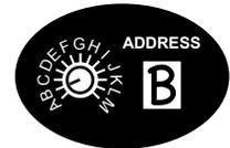
Address setting for the first 1176 in a stack (the AVatrix is addressed A).
