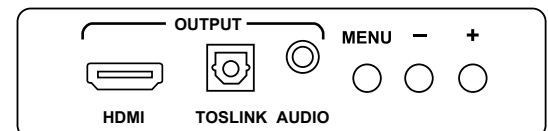
1385 outputs and user interface controls
