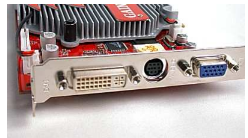
A typical computer graphics card, including a variety of video connections like DVI and VGA.
