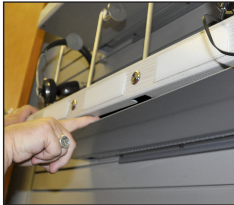
Screw shut the bottom of the Lower Shelf, checking for wires that may be pinched in the gap.
