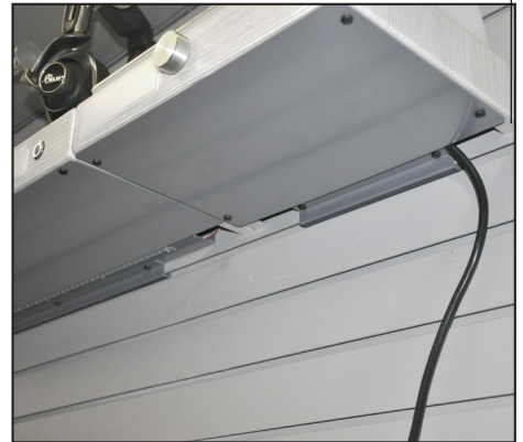
Attach the bottom cover to the Media Shelf with four screws provided. It may be helpful to clear each hole with a screw first, then install the panel.
