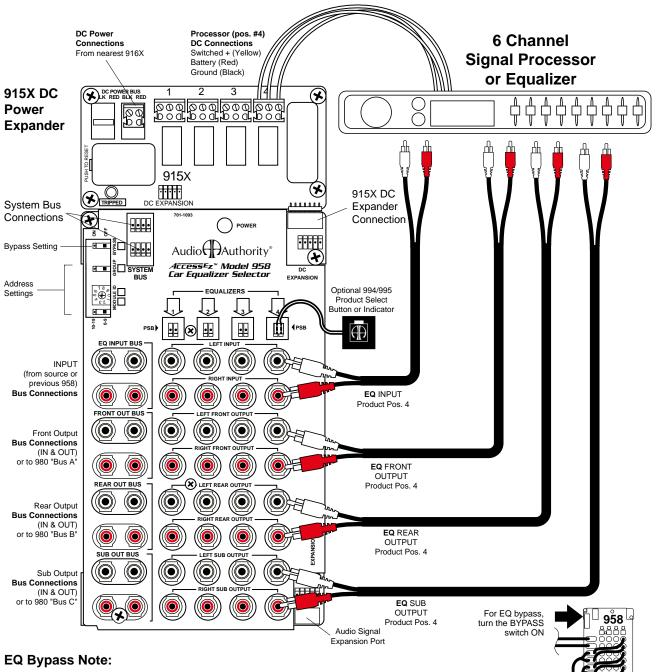
This EQ could not be connected in position #4 as shown if this were the last module in an Equalizer Product Group to be bypassed.
