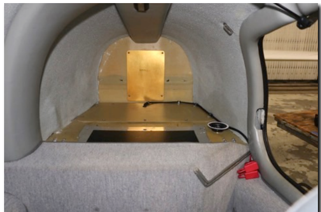
Aft baggage interior with trim removed.
