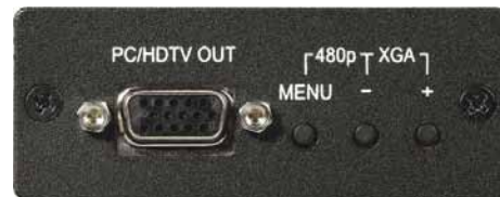
HD output (HD-15 connector) and adjustment controls
