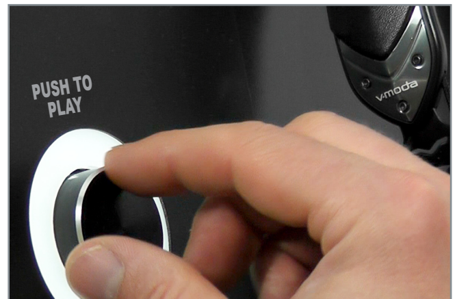
The Visual Volume knob provides a simple interface to adjust volume and play the next music track. The glow ring attracts customers with a slow pulse during attract mode, and visually indicates volume level during the demo. The knob is milled from aluminum for durability in retail environments.
