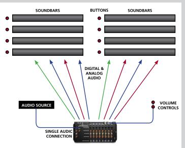
This system configuration switches up to eight soundbars using one audio source. Customers simply press the button next to each soundbar and adjust master volume using a knob.
