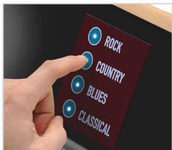
TouchSelect panels can be used in many different ways; in this case, each touch position activates the headphones, and simultaneously starts a music video in the genre selected.
