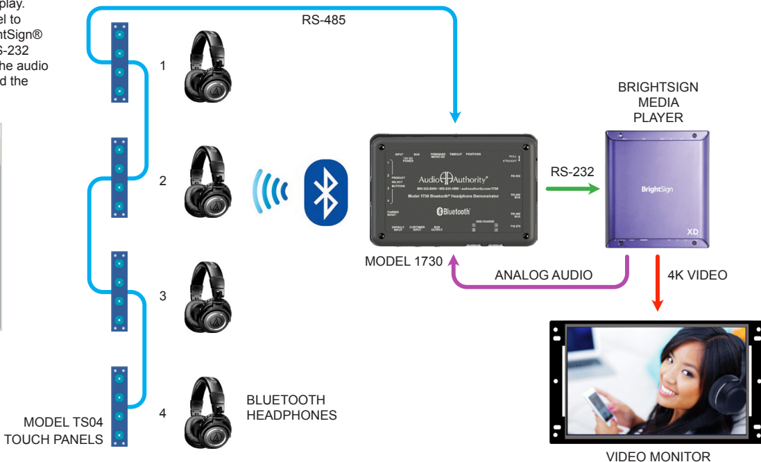
TouchSelect panels can be used in many different ways; in this case, each touch position activates the headphones, and simultaneously starts a music video in the genre selected.
