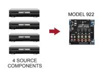
Switch up to four powered subwoofers with each 922 module.
