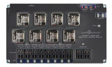
The Audio Authority® Model 939 answers to the demands of demonstrating higher-current speakers. The 939's half-inch board traces and huge relays can handle up to 2,500 watts per channel at 4 ohms, enabling it to handle even the most demanding applications for ear-splitting demonstrations. Use two 939's for stereo applications.
