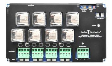
The Audio Authority® Model 939 answers the demands of demonstrating higher-current speakers. The 939's half-inch board traces and huge relays can handle up to 2,500 watts per channel at 4 ohms, enabling it to handle even the most demanding applications for ear-splitting demonstrations. Use two 939's for stereo applications.
