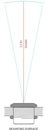
MOUNTING SURFACE MAX THICKNESS = 7.9 MM
