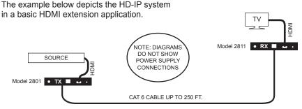
In this configuration, HDMI cables connect the source and display equipment to the respective 2801 Transmitter and 2811 Receiver. A Cat 5 or 6 UTP cable connects the 2801 to the 2811. Properly terminated Cat 6 cables will result in the longest possible range. Terminate the cables to either the EIA 568A or 568B standard for best performance. Correct pairing is vital, and should always be checked with a network cable tester. The DIP switches on the 2801 and 2811 should all be in the DOWN position.
