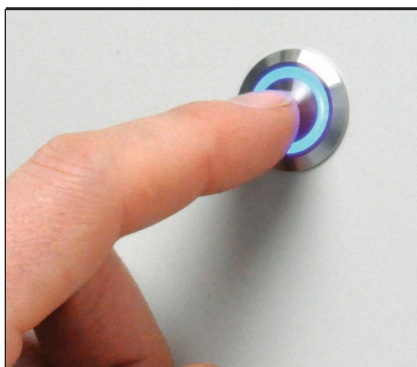
Figure 3. By pressing a Product Select Button (PSB) connected to a switching module.
