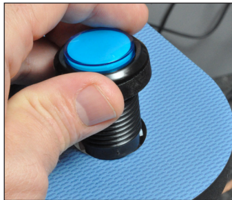
Figure 48. Plastic PSB button assembly.
