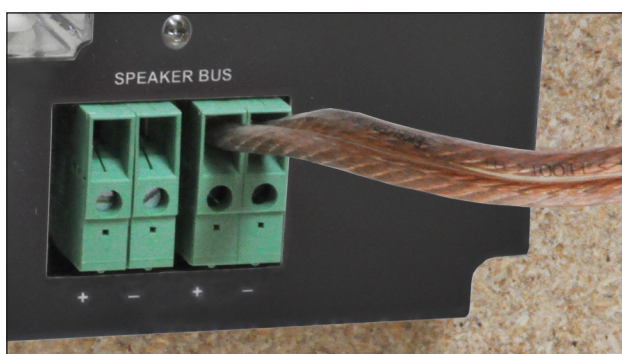
Figure 28. High-Power Speaker Bus using 12 gauge speaker cabling.
