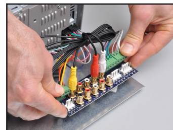
Figure 55. Mounting 9A15 to deck tray.
