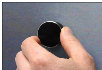
The 1894 Rotary Control knob rotates to control volume level and advances the track selection with a press. Available with a black or silver knob.
