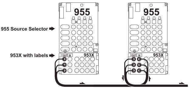
If 953X modules are to be used as expansion modules for component video on-screen display (as shown below) the module sending video to the receivers will use the printed legend. The video signal output from the receivers will connect to the 953X modules with labels applied over the printed legend.
