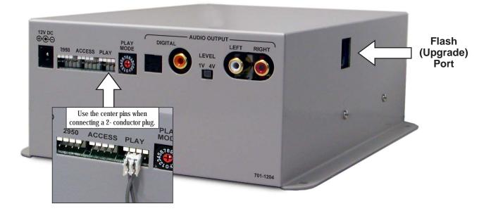
If the intended use of this player is as a source of 4-volt analog car audio, place the Level switch in the 4V position. For all other uses, leave it in the 1V position.
