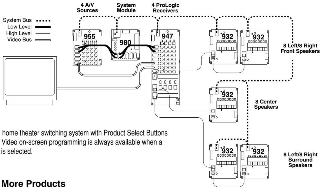
**Figure 15.** Small home theater switching system with Product Select Buttons by each product. Video on-screen programming is always available when a capable receiver is selected.
