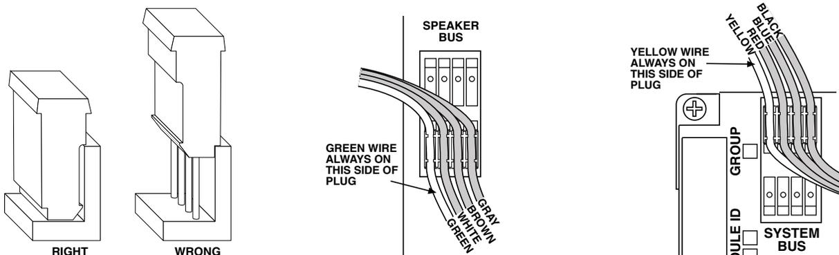
**Figure 37.** Check buses for polarity and solid connection.
