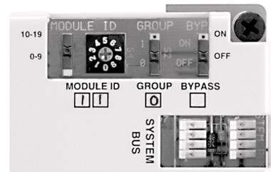
**Figure 23.** Source Module set to 0/11. Later, you will fill in the blank boxes with the settings for each address switch as shown.
