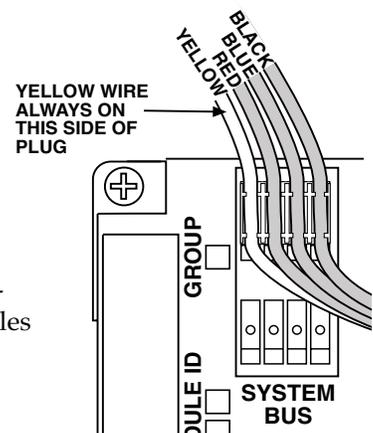
**Figure 28.** Observe correct System Bus polarity. It is fine to leave one header unused.
