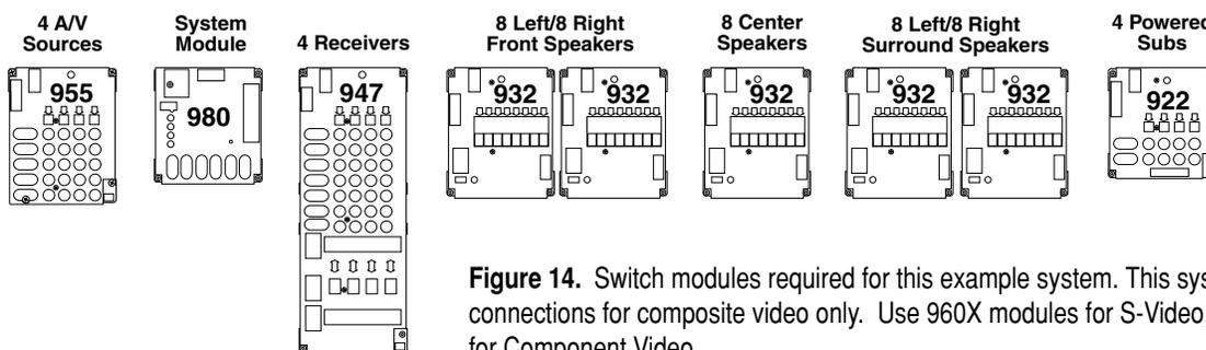
Figure 14. Switch modules required for this example system. This system has connections for composite video only. Use 960X modules for S-Video, and 954 modules for Component Video.
