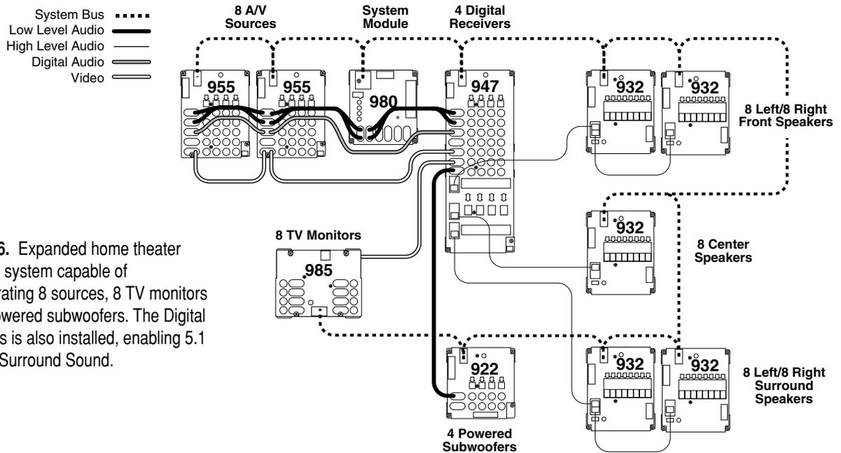
**Figure 16.** Expanded home theater switching system capable of demonstrating 8 sources, 8 TV monitors and 4 powered subwoofers. The Digital Audio Bus is also installed, enabling 5.1 Channel Surround Sound.
