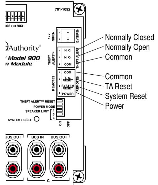
**Figure 43.** Headers available to connect remote power switch, a remote TheftAlert reset, and an alarm or siren for TheftAlert.
