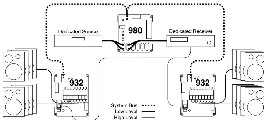
Figure 8. All modules are connected by system bus.
