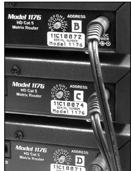
Note: If you are installing expanders on Model 1156 or 1166 the address scheme is different. Refer to the AVX-561 or AVX-661 manual.
