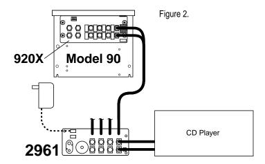
2961 power may be backed up, if desired, by an ordinary non-rechargeable 9-volt alkaline battery. Plug the battery into the battery socket in the corner of the 2961 module. When using battery backup, be sure that the 2961 remains powered from the AC wall outlet at all times, even at night, to prevent draining the battery. Install the releasable cable tie to discourage tampering with the battery. Release the cable tie to replace the battery. In systems, each 2961 must have its own backup battery.
