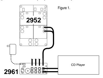
Borrow DC power for the 2961 from any Audio Authority digital switching system, or power the 2961 from a power pack such as Audio Authority part number 805-002. When borrowing power from a switching system, plug one end of the short bus cable supplied into the 2961 header labeled Bus. Plug the other end into the nearest 2950 System Bus header or one of the power headers of the Model 90.
