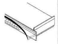
Packed with each Model 510 is a set of self-adhesive Lexan® panel inlays for indicating the type and number range of video components connected to it. For each Model 510:
