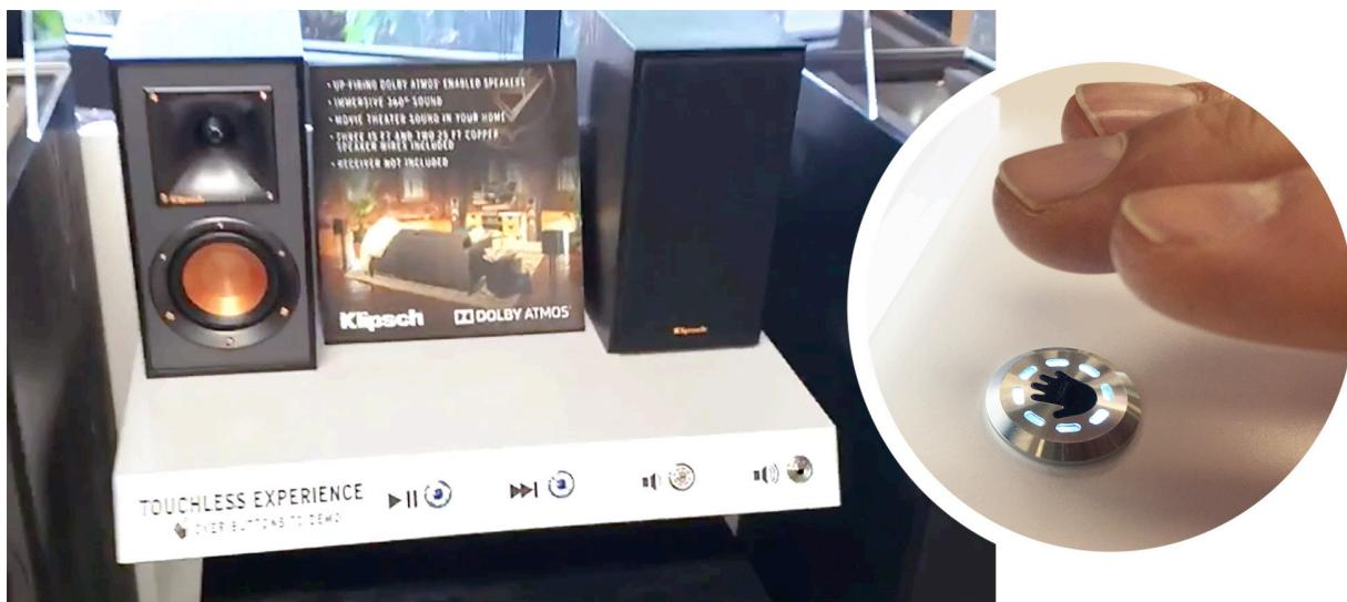
New Klipsch Audio displays use AirSelect touchless sensors by Ascentic Retail Engineering to protect consumers from the spread of pathogens. The hand symbol invites users to interact without touching, and response lights confirm the user's actions.
