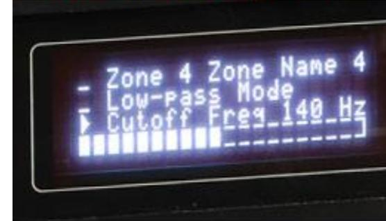
It's easy to add passive subs in all your zones with the SonaFlex matrix amplifier. Each 2.1 channel zone has its own low-pass filters and zone volume controls.
