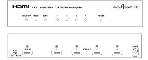
The 1394A has a single HDMI input and four HDMI outputs. The 1398A has eight outputs. The Power LED indicates that the unit is receiving power.
