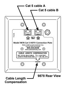
For example, if the coaxial cable length from main system to Driver is 220 feet (1 click) and the Cat 5 cable length to a certain Wallplate is 250 feet (2 clicks), the correct Cable Length Compensation for that Wallplate is 1 + 2 = 3 clicks.
