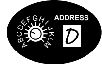
Address Setting for the fourth 1176 in a stack.
